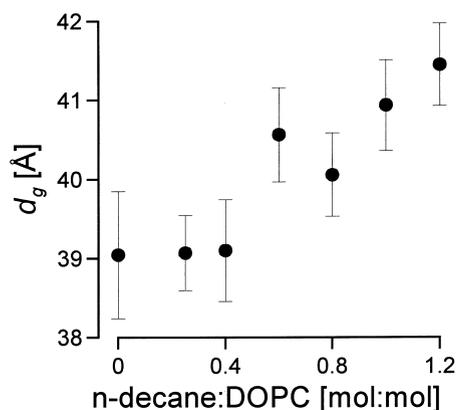
Fig. 3. Dependence of the DOPC bilayer thickness parameter  $d_g$  on the *n*-decane/DOPC molar ratio.
