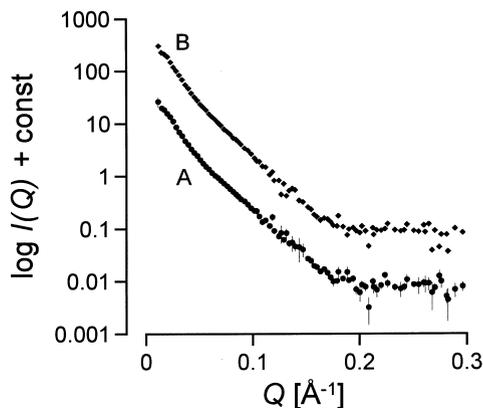
Fig. 1. The dependence of SANS intensity  $I(Q)$  on the scattering vector  $Q$  for extruded unilamellar DOPC liposomes in the absence (a) and presence (b) of *n*-decane (molar ratio *n*-decane/DOPC = 1:1). The dots indicate the mean values obtained by averaging over seven circular detectors and the error bars the S.E. of the mean value.
