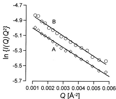
Fig. 2. Kratky–Porod plots of neutron scattering curves for extruded DOPC liposomes in the presence of  $n$ -decane at molar ratios  $n$ -decane/DOPC of 0.25:1 (curve A, diamonds) and 2:1 (curve B, circles).
