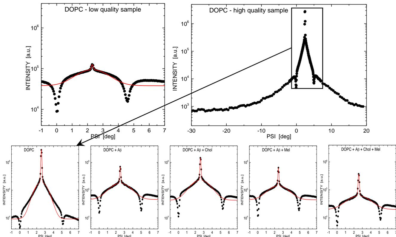
**Figure 1:** Uncorrected rocking curves measured for various samples investigated in the experiment. The diffraction intensity is collected as a function of the sample angle PSI, while the detector active area is fixed at the position of the first diffraction order.<sup>8</sup>
